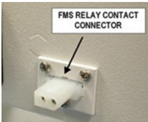
Figure 8. FMS Relay Contact Connector on Rear Panel
