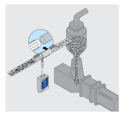
Remove static charges generated on plastics by installing a Conveyostat before and after the cyclone to keep the material moving freely.
